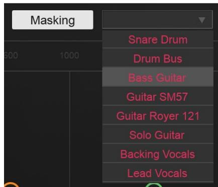
The Masking Meter displays momentary indications of masking—loudness loss—as vertical white lines over the current track’s spectrum and EQ curve (we affectionately refer to this meter as the “Northern Lights”!). These lines indicate that there was some amount of loudness loss at that frequency at that moment: the brighter the line, the greater the masking amount.
